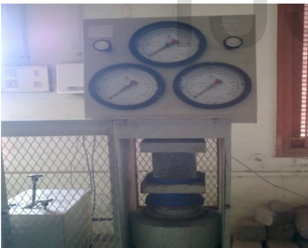
Fig 1. Specimen in compressive testing machine (cube)
