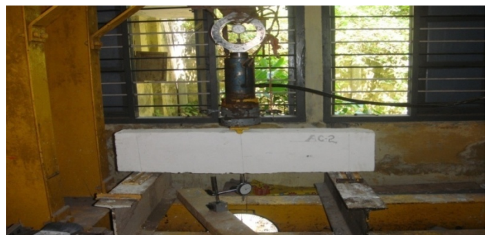
Fig. 5. Static load set up for beams
